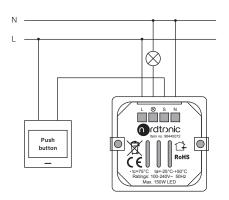
Multiple push switches wiring for multiple control points
